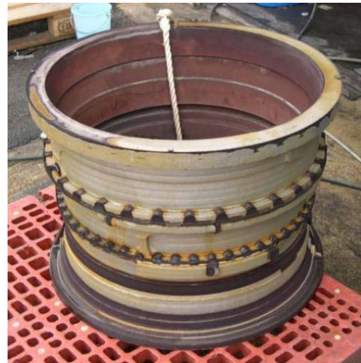
Figure 4: Net-Shape Ti6/4 Powder HIP'ed V2500 Front HP Compressor Casing. Figure 5: Mild Steel Tooling Partially Dissolved from Powder HIP'ed V2500 Casing.
