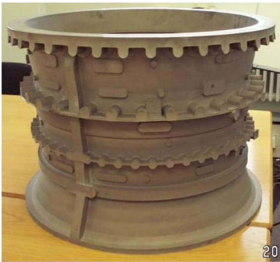
Figure 4: Net-Shape Ti6/4 Powder HIP'ed V2500 Front HP Compressor Casing. Figure 5: Mild Steel Tooling Partially Dissolved from Powder HIP'ed V2500 Casing.
