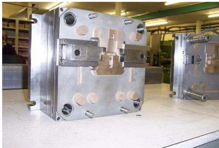
Figure 11: Powder Bed Laser Processed MIM Tooling for a 316L Stainless Steel Stator.
