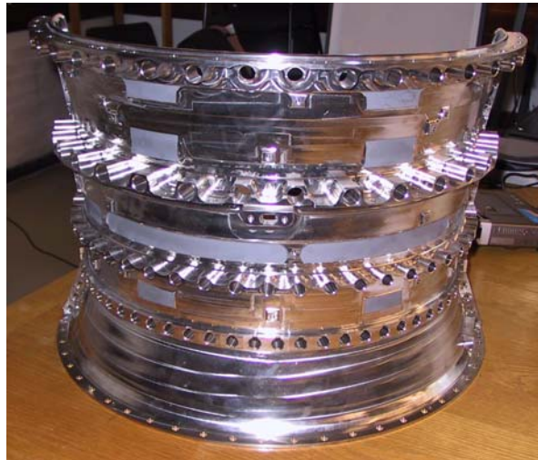
Figure 3: V2500 Front HP Compressor Casing Machined from a Ring-Rolled Forging.
